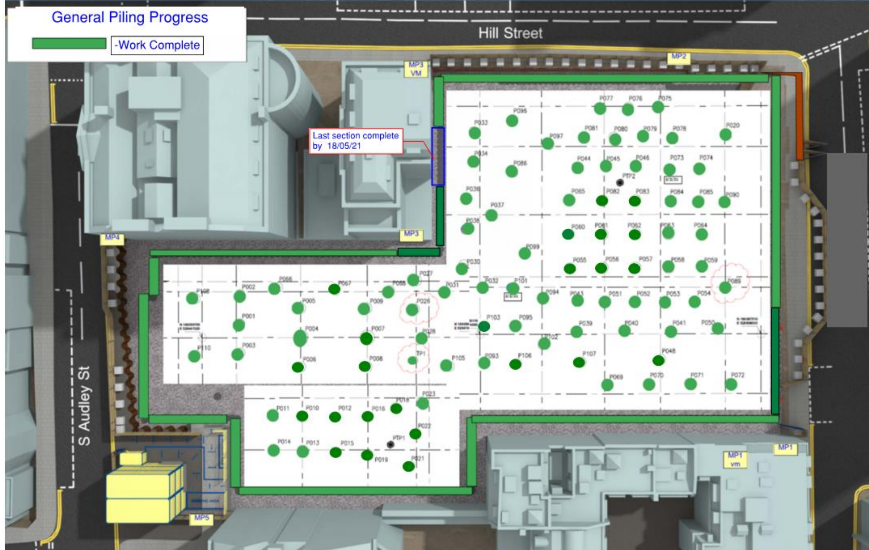
Layout highlighting Piling Complete
